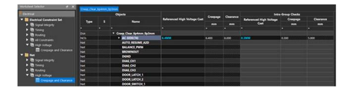
Creepage: Distance measurement along surface of material between high-voltage objects.
