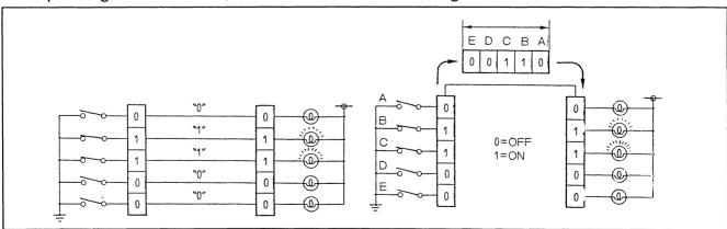
Serial communication is mainly used between the A/C amplifier and the information display. All display signals can be sent by only 4 signal conductors.
