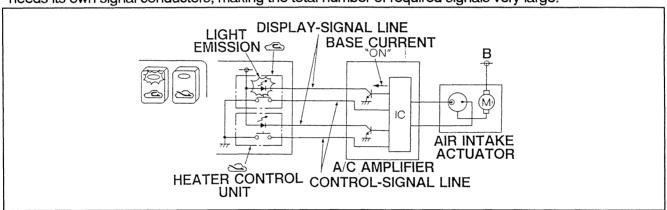
As for the Full Auto Air Conditioner, to prevent increasing the number of signal conductors, information interchange is done between the heater control unit and A/C amplifier by serial communication. Normally, to turn on each light, each signal conductor is needed. However, serial communication can be used to send plural signals. Therefore, we can reduce the number of signal conductors.
