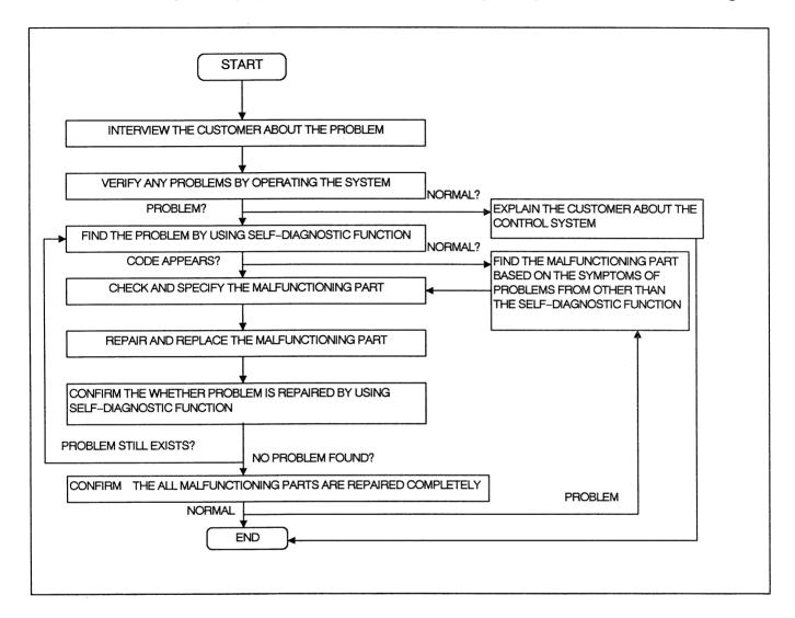
The most important point in troubleshooting the auto air conditioner is to try to find the cause logically based on customer interview or by the result of the self-diagnosis function, and then to repair the problem. Furthermore, you should confirm whether the problem is repaired completely or not.
