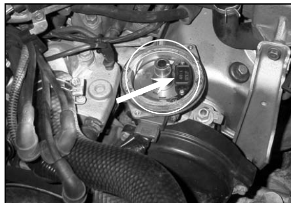
Crank angle sensors on engines with distributors are usually located within the distributor.
